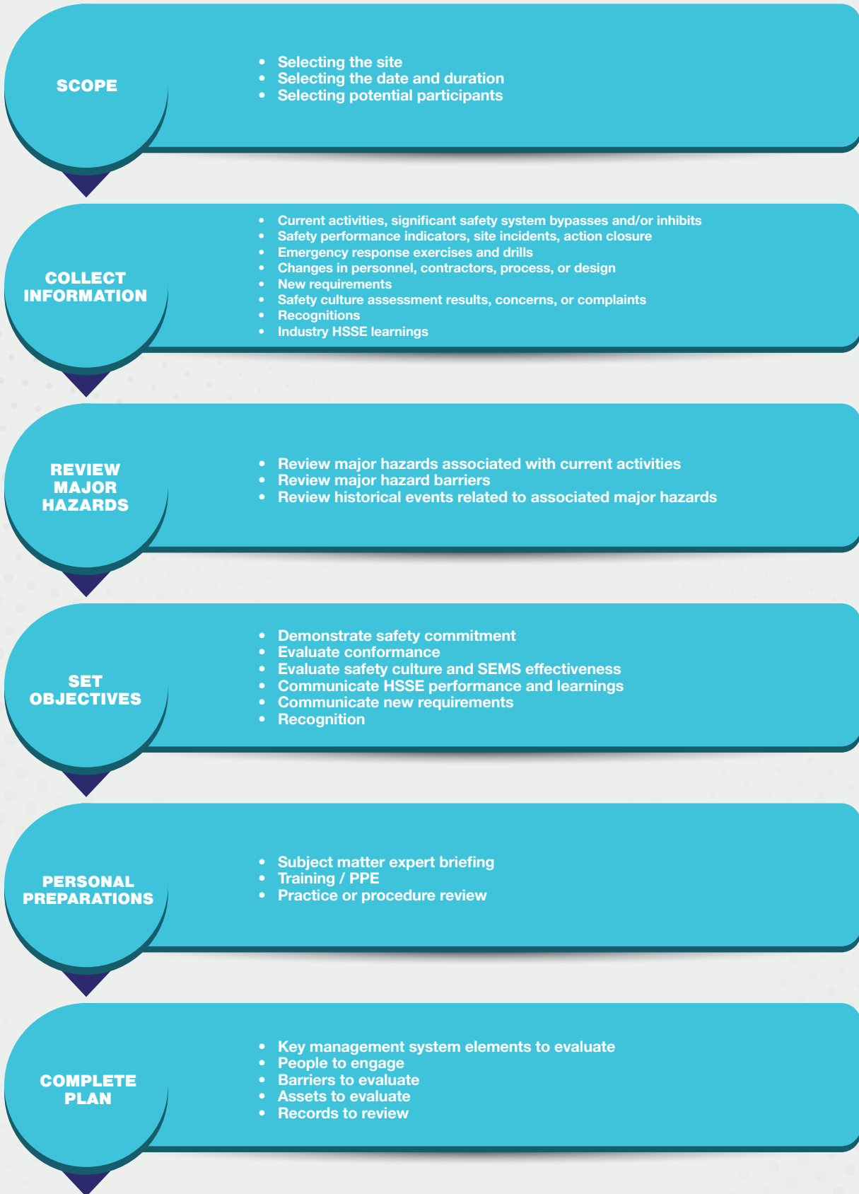
FIGURE 4—LSE PREPARATION STEPS
